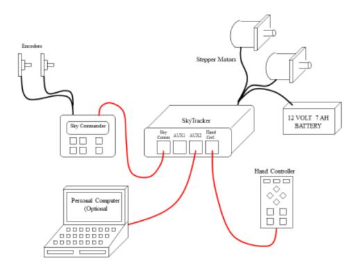
Figure 1 SkyTracker Wiring Configuration
