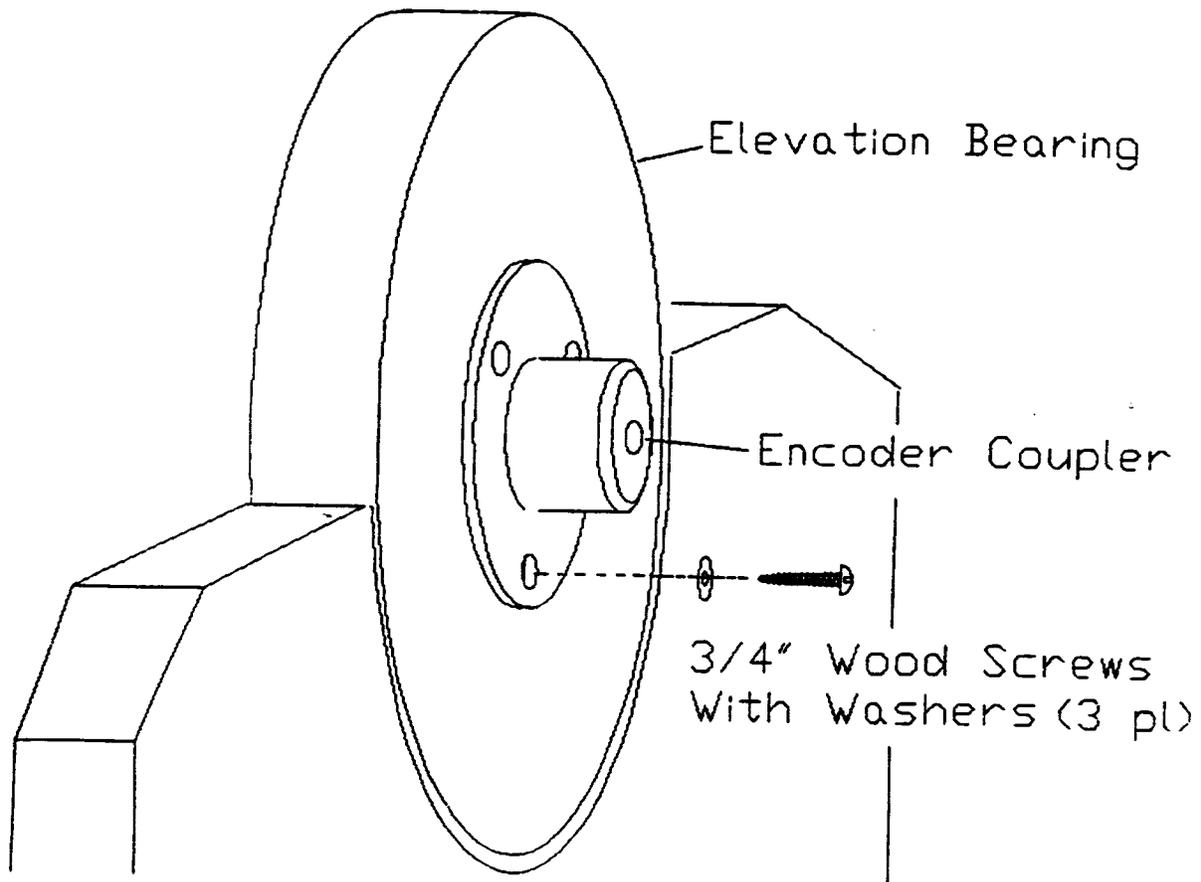
3. Install the elevation encoder/tangent arm assembly by sliding the forked end over the anchor pin and then inserting the 1/4" shaft of the encoder into the hole in the coupler. Tighten the nylon thumb screw.
